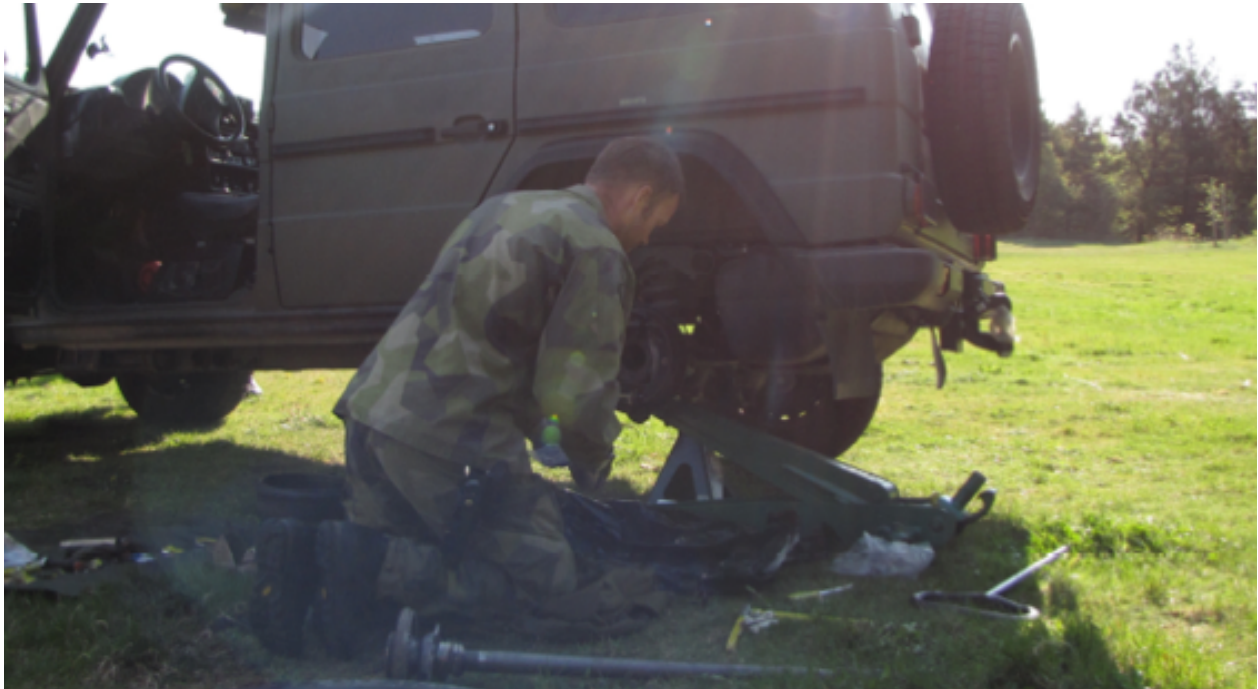
Picture 4: Replacement of wheel on a Swedish vehicle in the field. 99
