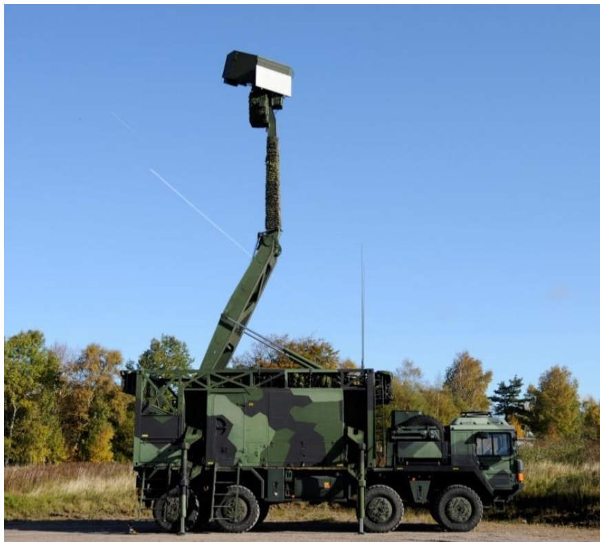
Figure 1. The Giraffe AMB radar which can be used to detect and track airborne platforms, © Saab AB, Photograph: Peter Liander
