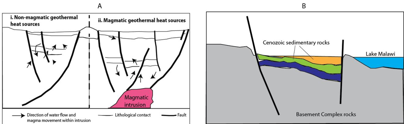
**Figure 4: Proposed schematic section across the Karonga area of the Malawi Rift, Northern Malawi (after Manzella, 2009).**
