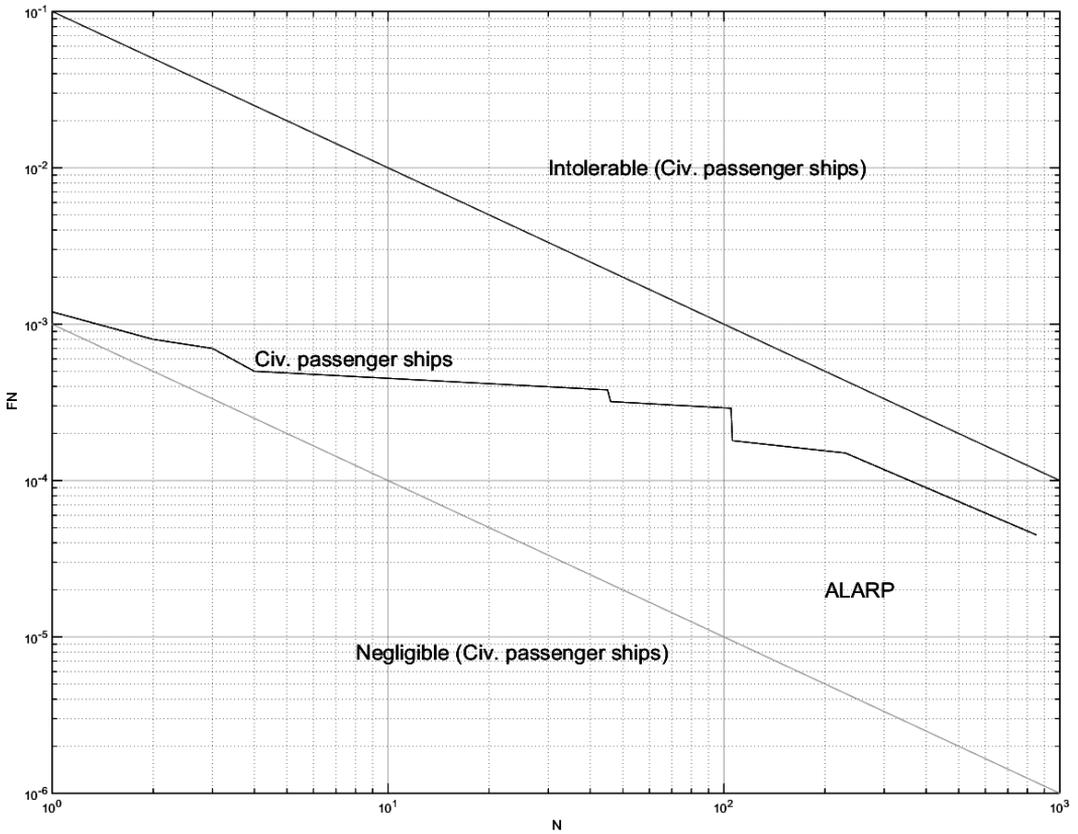
Figure 1. FN-diagram showing the societal risk per ship year in relation to the number of fatalities for passenger ships worldwide for the years 1989–1998. Data and limits according to IMO.<sup>41</sup>
